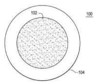
A molded contact lens comprising a stiffer optic zone relative to the peripheral zone of the contact lens provides an optical element for correcting astigmatism without the need for or substantially minimiz-
