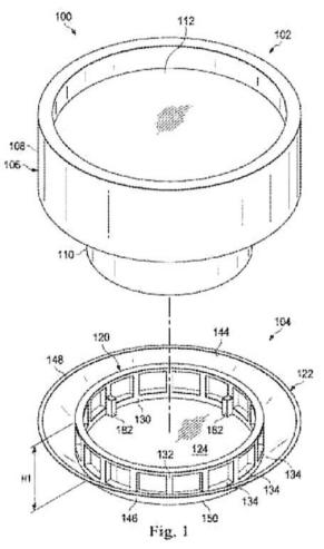
A lens holder (104) for holding a vitrectomy lens (102) during a surgical procedure, comprising: a support ring (120) sized and shaped to receive a portion of a vitrectomy lens to provide visualization of a surgical site in an eye of a patient, the support ring being configured to rest upon the eye of the patient during a surgical treatment procedure performed on the eye; a transparent, flexible membrane (124) disposed along a bottom plane of the support ring, and configured
