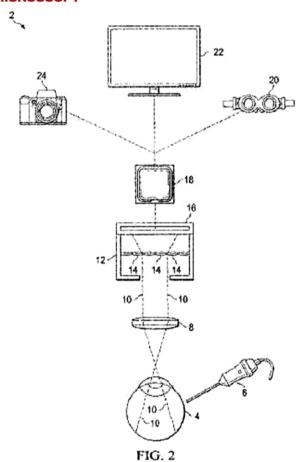
A system and method for ophthalmic surgery in which a light field camera is used to capture a digital image of the surgical field including the eye. The digital image is used to create image information and directional information, which is then used to from a three dimensional (3D) image with motion parallax.
