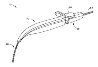
An apparatus for delivering therapeutic agent to an eye comprises a body, a cannula, a hollow needle, and an automated actuation assembly. The cannula extends distally from the body and is sized and configured to be insertable
